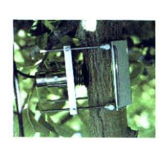
Our OEM makes an adapted fixture to fix the LVDT directly on the samples. The tests could be also engaged directly on the field, everywhere on the globe. The communication will be handled by a low power consumption electronics, including a GPRS transfer mode.
